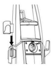
**3. Installing the power cord hook into position of unit right**
