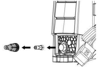
Clean the nozzle with the needle cleanout tool provided . Remove the spray wand from the gun. Remove any dirt from the nozzle hole and rinse.
