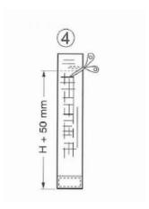
2. Cut each piece according the height H + 50mm
