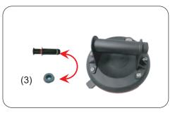
2. Loosen the bolt from the piston body, remove washer, replace the sealing ring (3). Insert the washer and secure with the screw
