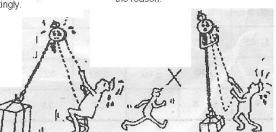
8. In case of the hand chain fails to move, don't pull it violently or by increasing force. Stop operation and look for the reason.
