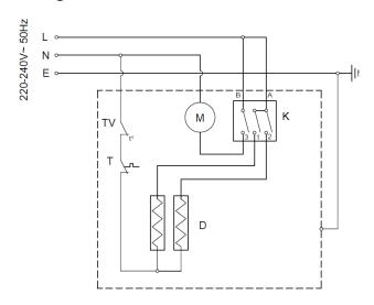
T: Thermostat K: Switch M: Motor D: Heating element
